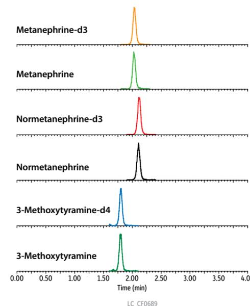
**Even at 50 pg/mL, good signal-to-noise ratios mean lower LOQs and accurate results at trace levels.**
