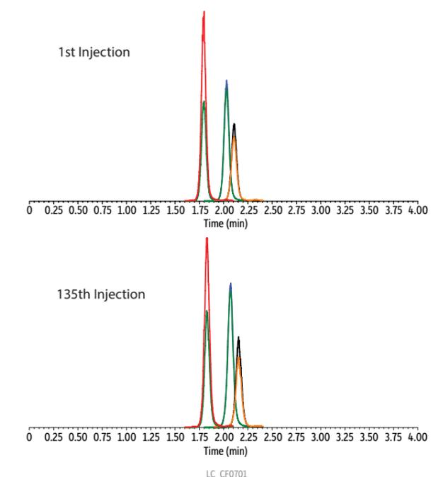
Column: Raptor HILIC-Si (cat.# 9310A52); Dimensions: 50 mm x 2.1 mm ID. Particle Size: 2.7 µm; Temp.: 30 °C; Sample: Diluent: Mobile phase A:mobile phase B (10:90); Conc.: 1 ng/mL; Inj. Vol.: 10 µL; Mobile Phase: A: Water, 100 mM ammonium formate, pH 3.0; B: Acetonitrile; Gradient (%B): 0.00 min (90% B), 5.00 (90% B); Flow: 0.3 mL/min; Detector: MS/MS; Ion Mode: ESI+; Mode: MRM; Instrument: UHPLC
